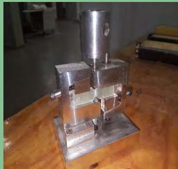
Specimen testing jig machined from stainless steel.
