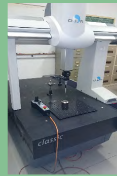
Co-ordinate Measuring Machine (CMM) accurately measures components for reverse engineering
